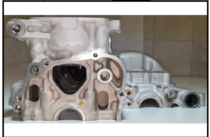
C3-6) Bloc-cylindre nu vu de côté Admission Bare cylinder block seen from intake side
