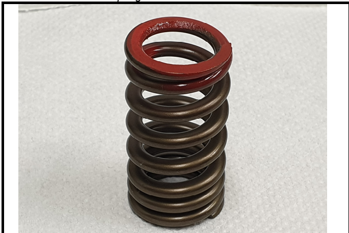
C10-8) Ressort soupape admission Intake valve spring
