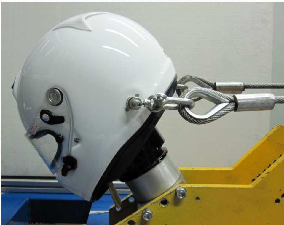
Figure C2. Appareil d'essai des Fixations de Casque M6 (casque d'essai installé) (1) / Figure C2. Apparatus for testing Helmet-M6-Terminals (with test helmet fitted) (1)
