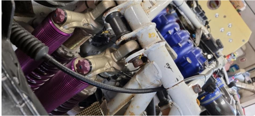
Routing of cable from actuator towards clutch pedal
