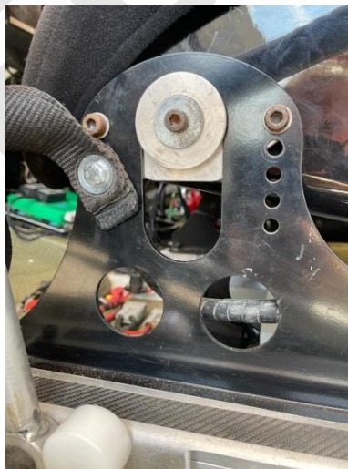
Leg strap attachment to the seat bracket
