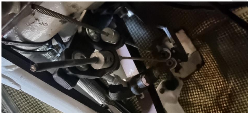
Clutch pedal with both cables attached (actuator + hand-lever)
